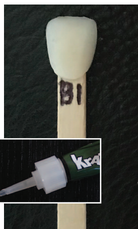
Fig. 3.2–3.3: Glue the cured composite to a wooden handle and mark the shade
