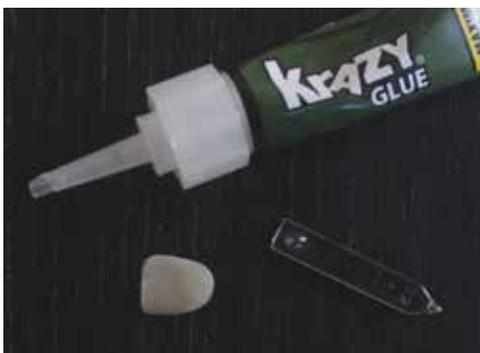
Fig. 5: Composite shell is removed from the template and glued to a handle.
